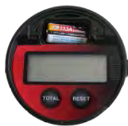
Picture 2: Take out the battery
