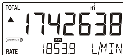
Fig. 4: Example of low-battery alarm.
