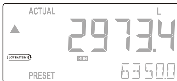
Fig. 6: Example of low-battery alarm.
